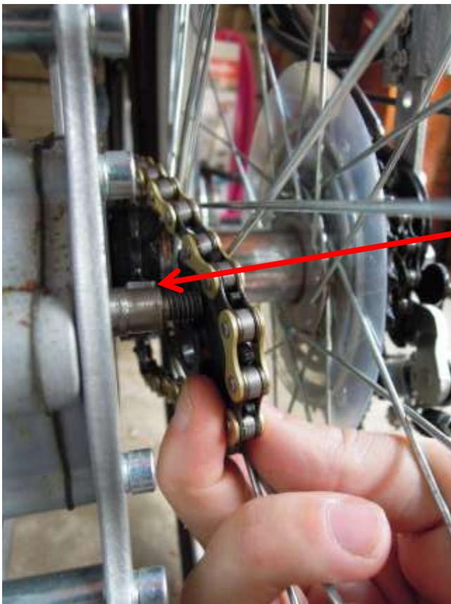
**This is the pin. It can and will fall out. Line this up with the notch in the sprocket while keeping it in place. This was the most challenging part of the modification.**
